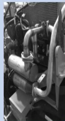
Modified Exhaust System
