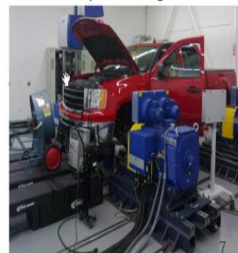
Gasoline Passenger Vehicle Chassis Dyno Testing
